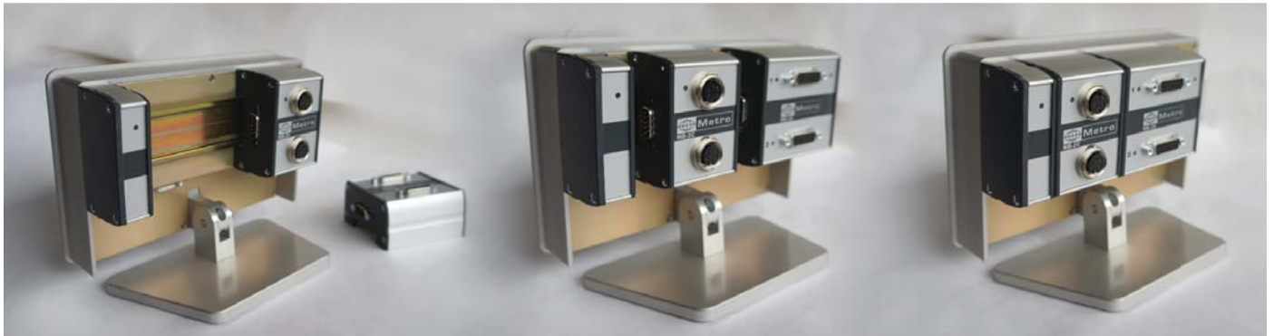
Installation of the first module
