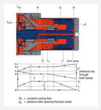
The cooling flow is led from the discharge side behind the impeller into the chamber between the slide bearings and through the pump shaft via the rotor back vanes again to the discharge side. This design pressurizes the slide bearings and the containment shell with nearly the full discharge pressure and the product remains stable in this area.
