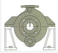
The casing forms - together with the containment shell - the pressure retaining pump unit. Maximum allowable pressure at PT is determined by the shell design and the material. The pump casing has metal-to-metal fits with confined compression controlled gaskets.
