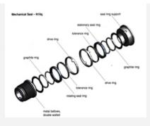
The "N10q" seal with metallic bellows and auxiliary gland packing according to DIN 4754 is available as standard in the NKLs-HTM pumps. The design with rotating double walled bellows and proper designed wear resistant mating faces of SiC ensures a long service life, also for pumping hot oils containing some solids like coke particles and pipe scale. The rotation of the bellows and the conical shape of the seal chamber avoids clogging and seizing of the bellows.
