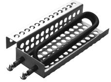
WATROD™ enclosure heaters are designed to prevent freezing and condensation in electrical and mechanical housings. The WATROD element is enclosed in a perforated, aluminized-steel bracket to prevent direct contact with heating element.
