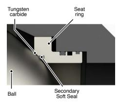
The secondary seal is the soft seal that allows the valve to seal when there is low pressure in the system; it also provides a seal that prevents sludge or foreign material from being trapped between the annulus and plug.
