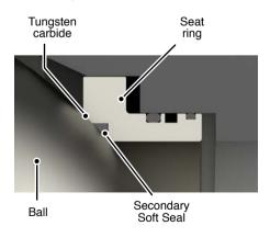
When the pressure decreases again, the soft (secondary) seals return to their position due to the phenomenon of resilience. This dual-action provides a tighter seal for longer and fewer in-service problems.
