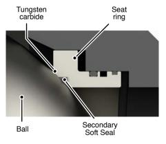
When the pressure increases, the soft seals collapse in their elastic zone; then the metal coating (primary seal) of the ball comes in contact with the metal seal of the seat rings achieving the metal-to-metal seal.
