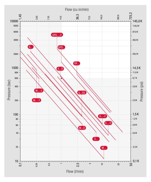
The performance data indicated here were determined with optimal flow cross-sections and the required volume flow for driving air.
