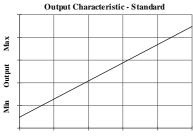
Retracted Linear Displacement Extended
